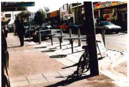
BARKLY STREET - given the narrow width of the footpath, the space would be improved by removing the furniture and bicycles from the path onto the outstand, as shown here in the existing kerb extension
